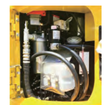
Fuel Feed Pump
